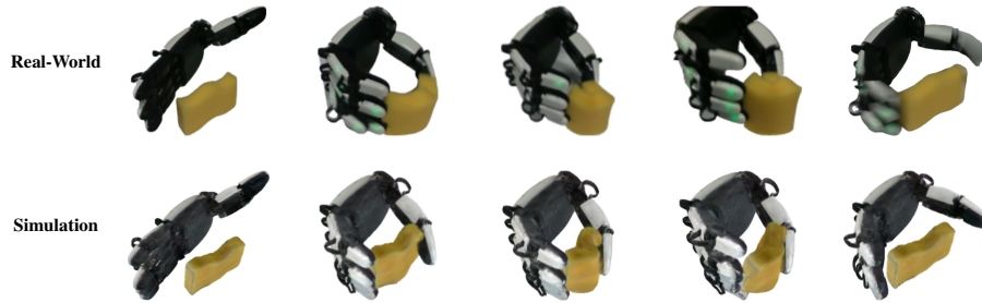
Figure 3. We perform dexterous grasping of a soft object (a sponge) in both the real world and in simulation. The physical parameters are empirically set and may not align with real-world conditions. The discrepancy between simulation and reality arises from both initial state biases and limitations in the physical model.
